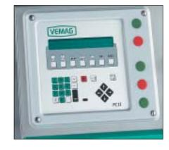
with ergonomics in mind. Up to 99 programmes can be stored. The operator enters the nominal values at the ten-character keypad of the portioning computer and conformation is by pressing a single key. Weight corrections can be entered directly in grams. All output information is displayed as clear text in the desired language. The portioning computer can be linked by the VEMAG Online net programme package to a central computer in the plant and – in a further extension to the system – via a mo-
